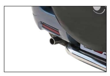
EM/240/IX End muffler Ø 50 mm
